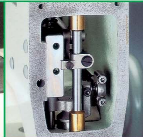
针柱固定滑板之设计，使针柱不易晃动，压脚心结构改良。 The needle fixator keeps the needle from vibration while the platen core comes with a modified mechanism.
